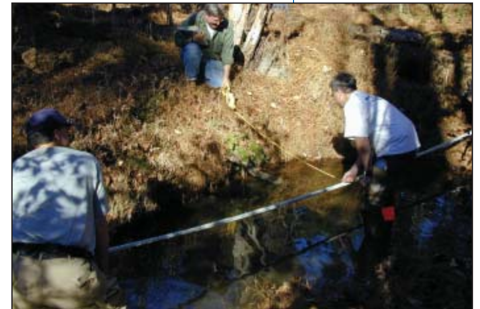
Figure 2.8 Field measurement of radius of curvature
