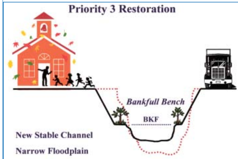
Figure 5.4 Cross section of a Priority 3 restoration project
